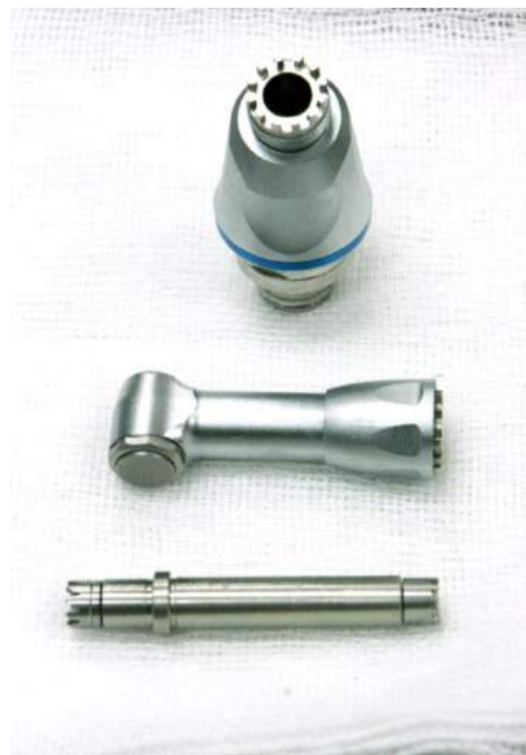
4) Remove oil completely by using tissue or gauze and install them again
